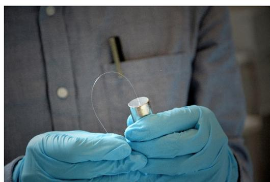
Experimental setup consisting of an 18650 cell and optical fiber “Bragg” grating (FBG) sensors.
